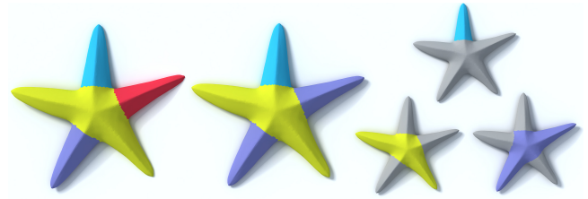
(a) Part count reduced from 4 to 3.
