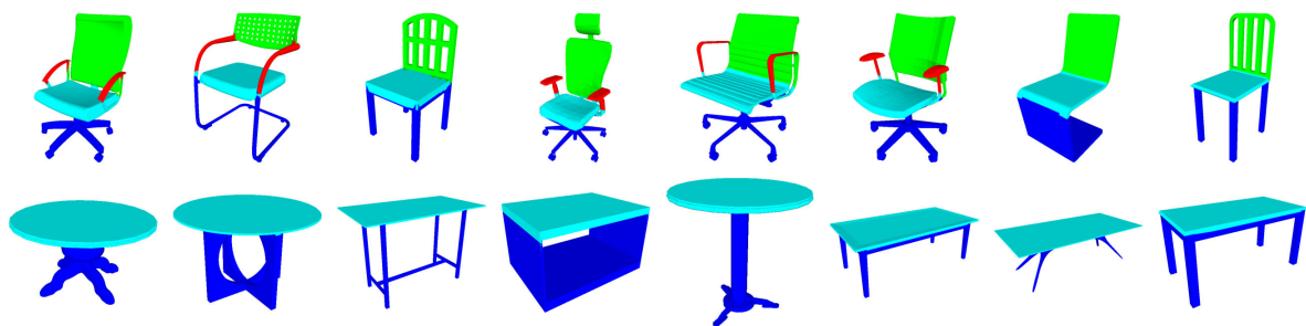
Figure 5. Unsupervised segmentation results on a joint set of chairs and tables from ShapeNet Part dataset.
